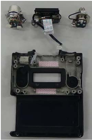
Fig.17:Remove the MIC/ANTENNA connector and RM assembly
