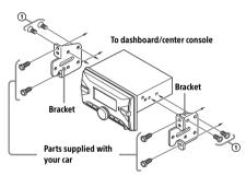
When mounting this unit to the preinstalled brackets of your car, use the mounting screws 1 in the appropriate screw holes based on your car: T for TOYOTA and N for NISSAN.
