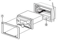
If the catches are straight or bent outwards, the unit will not be installed securely and may spring out.
