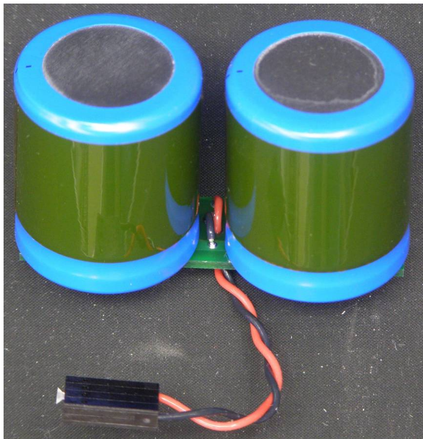
Figure 12 – Power Storage Assembly
