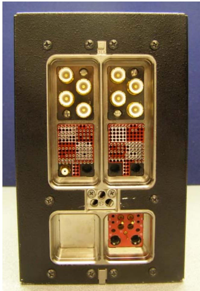
Figure 4 - Rear View, Detail of MCU Connector
