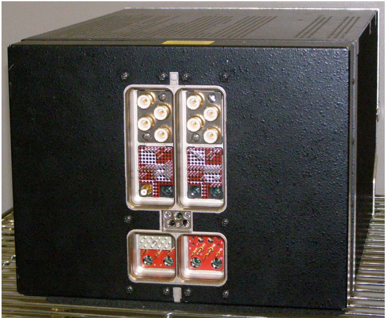
Figure 4 - Rear View, Detail of ARINC Connector
