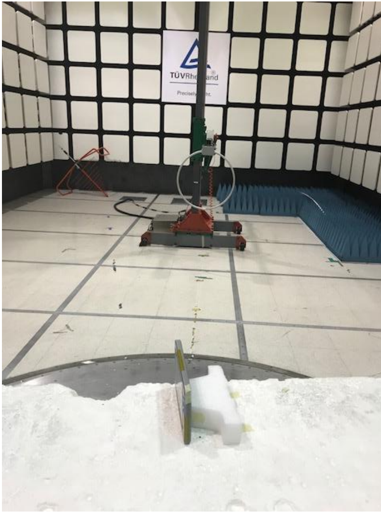
Figure 27: 9 – 30,000 kHz Radiated Emission Test Setup – Front View
