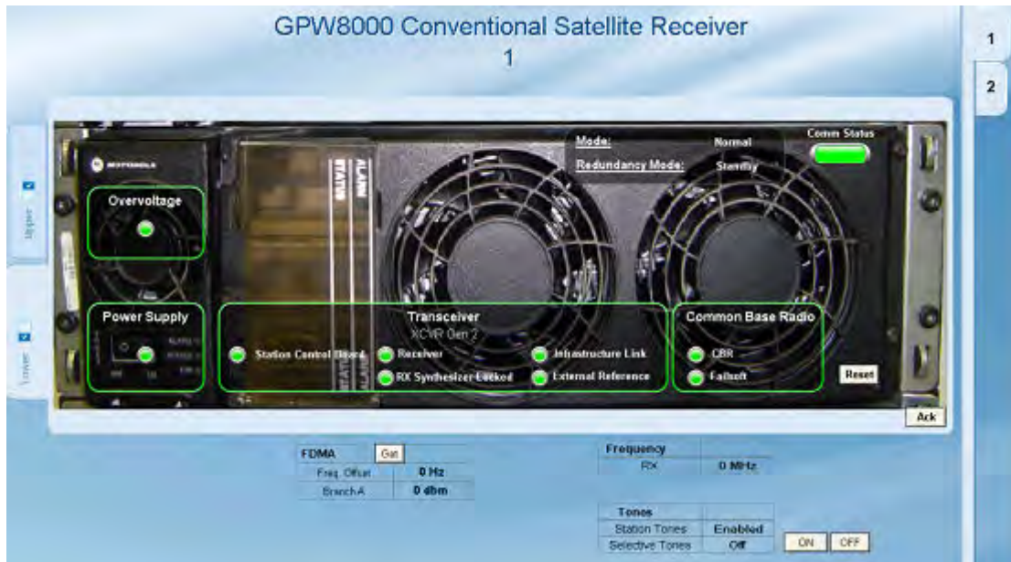
Figure 90: MOSCAD Network Fault Management – Example
