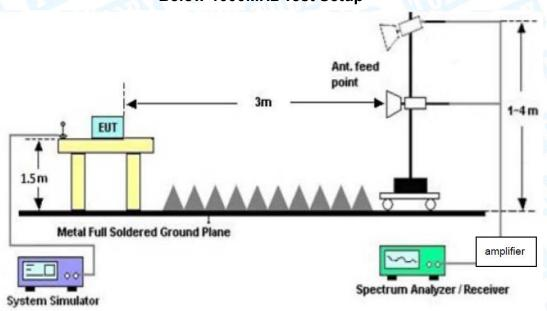
**Above 1GHz Test Setup**
