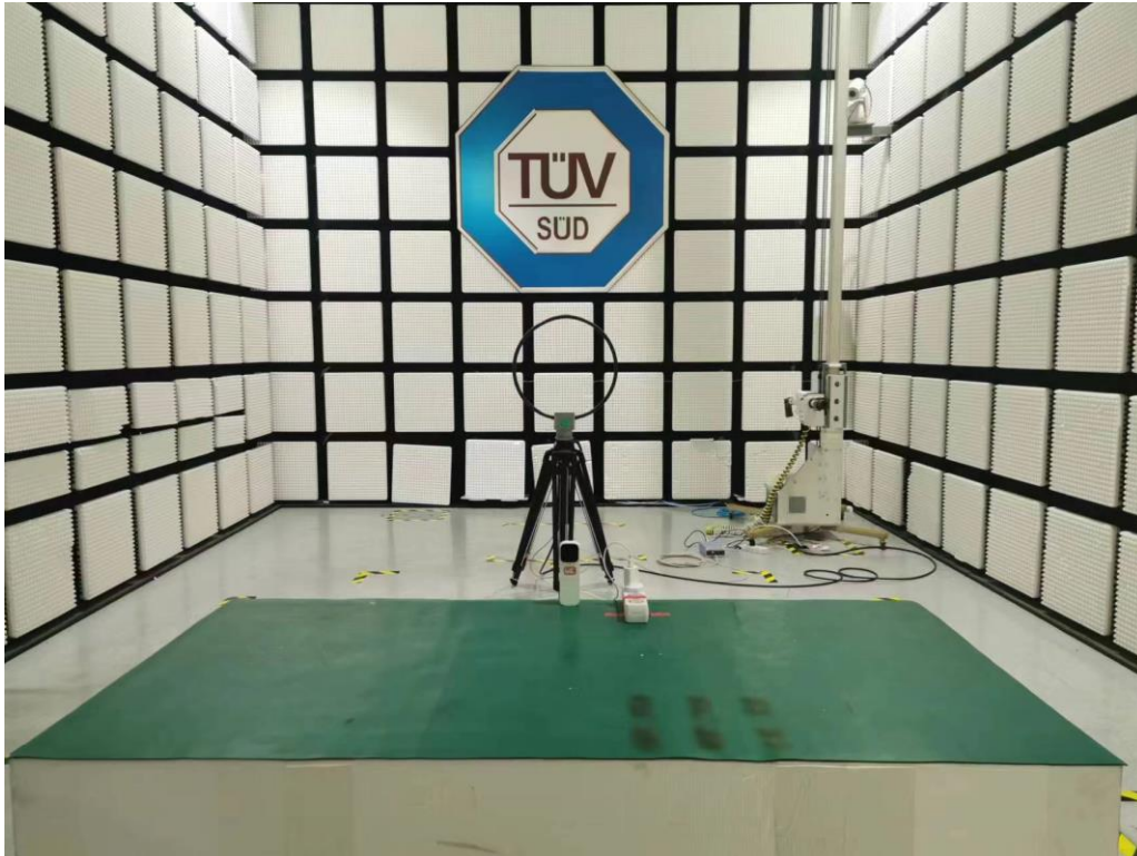
Radiated Emission Setup 9KHz-30MHz
