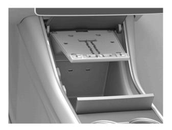
In 2021 and later models, plug in the K3Y in the glovebox USB port
