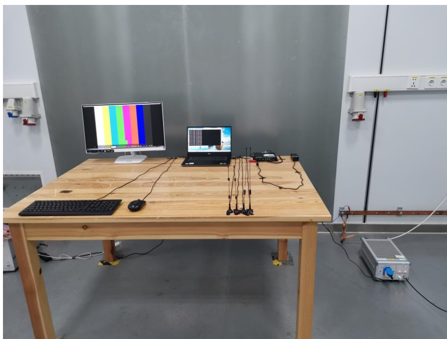
Fig. 4 Power line conducted emission setup photo
