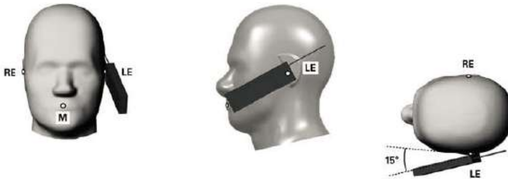
Fig.11.4 Illustration for Tilted Position
