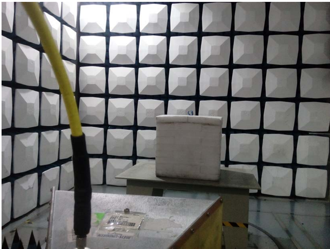
Radiated Emission Above 1GHz View
