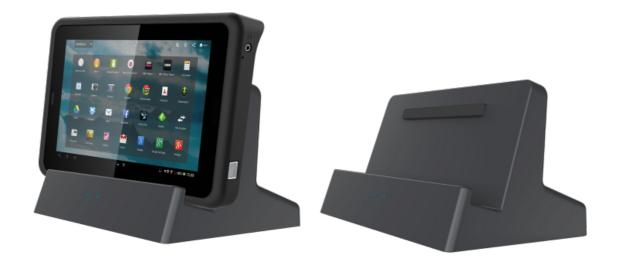
Use only the docking station included with your Tablet PC. Using other docking stations may damage the device.
