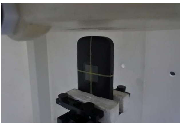
Bottom Side, Test Separation 10 mm
