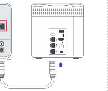
2. If using a combination modem/router, connect the other end to LAN port
