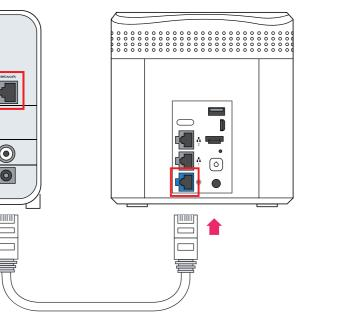
2. If using a combination modem/router, connect the other end to LAN port.
