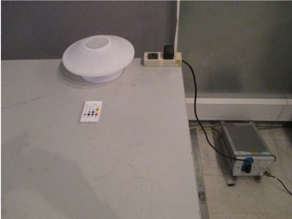
Measurement of Conducted Emission Test Set Up
