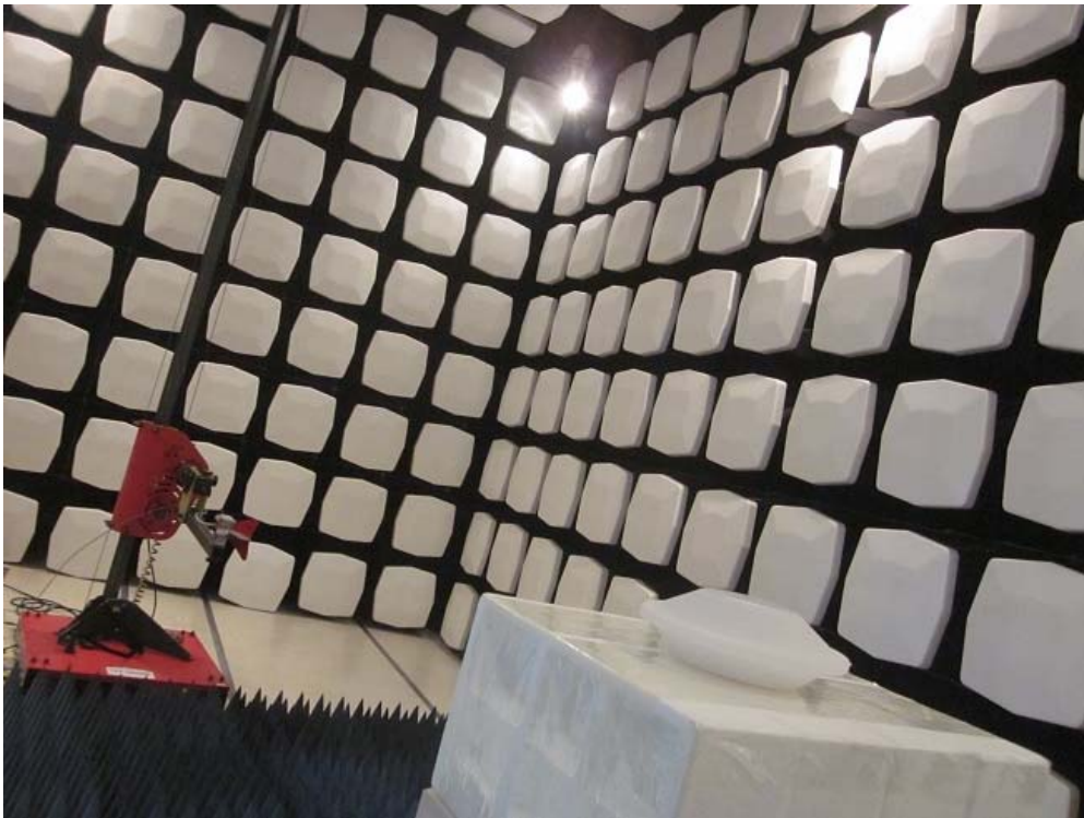
Measurement of Radiated Emission Test Set Up
