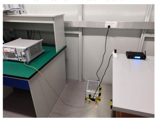
FCC RADIATED EMISSION TEST SETUP BELOW 1GHZ
