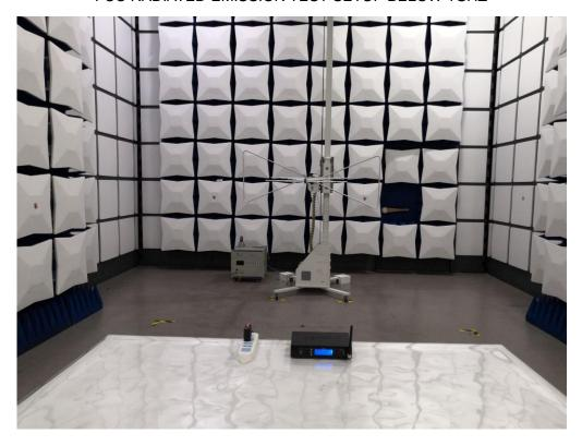
FCC RADIATED EMISSION TEST SETUP ABOVE 1GHZ
