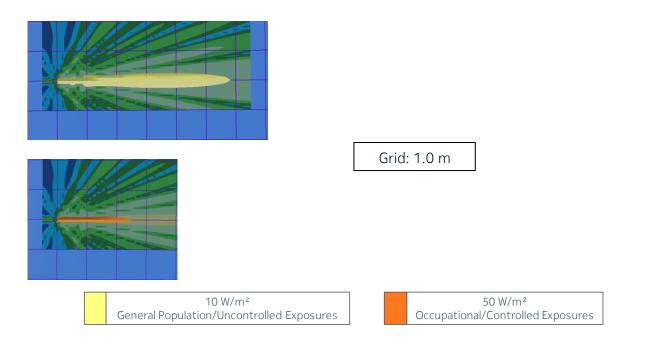
Figure 3 – Power density from AWKUC/D for the actual maximum transmitted power of 4.2 W (corresponding to the actual EIRP threshold of 66.25 dBm) and the beam oriented in azimuth =  $0^{\circ}$  & elevation =  $0^{\circ}$  (top view)
