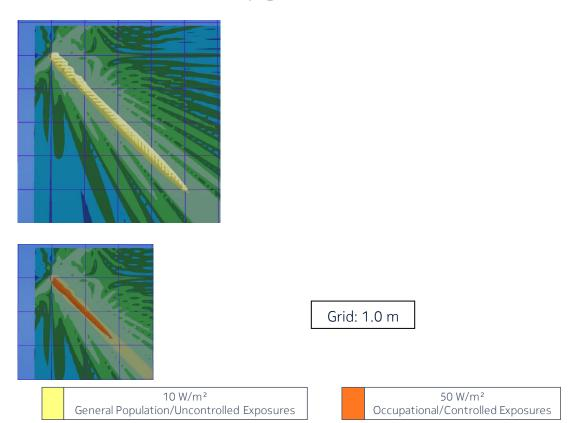
Figure 7 – Power density from AWKUC/D for the actual maximum transmitted power of 8.4 W (corresponding to the actual EIRP threshold of 66.25 dBm) and the beam oriented in azimuth =  $0^{\circ}$  & elevation =  $+45^{\circ}$  (side view)
