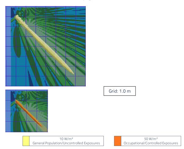
Figure 6 – Power density from AWKUC/D for the time-averaged maximum transmitted power of 16.8 W (corresponding to the time-averaged maximum EIRP of 72.25 dBm) and the beam oriented in azimuth =  $0^{\circ}$  & elevation =  $+45^{\circ}$  (side view)
