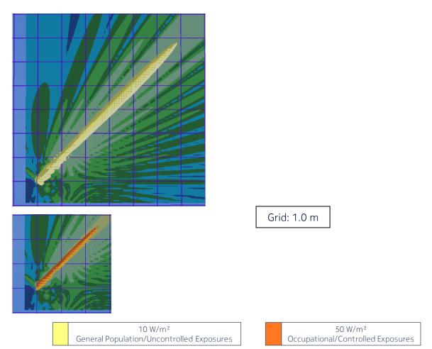
Figure 8 – Power density from AWKUC/D for the time-averaged maximum transmitted power of 16.8 W (corresponding to the time-averaged maximum EIRP of 72.25 dBm) and the beam oriented in azimuth =  $0^{\circ}$  & elevation =  $-45^{\circ}$  (side view)
