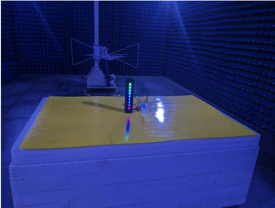
Photo of Radiated Emission Measurement Below 1GHz
