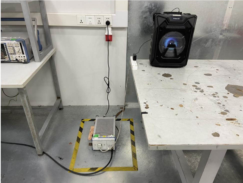
Photo of Power Line Conducted Emission Test
