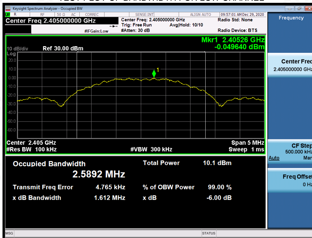
TEST PLOT OF BANDWIDTH FOR LOW CHANNEL
