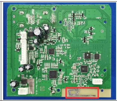
The antenna is PCB antenna. The best case gain of the antenna is 0dBi.
