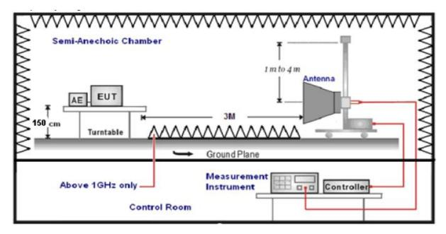
a. 1) Below 1G: The EUT was placed on the top of a rotating table 0.8 meters above the ground at a 3 meter semi-anechoic camber. The table was rotated 360 degrees to determine the position of the highest radiation.
