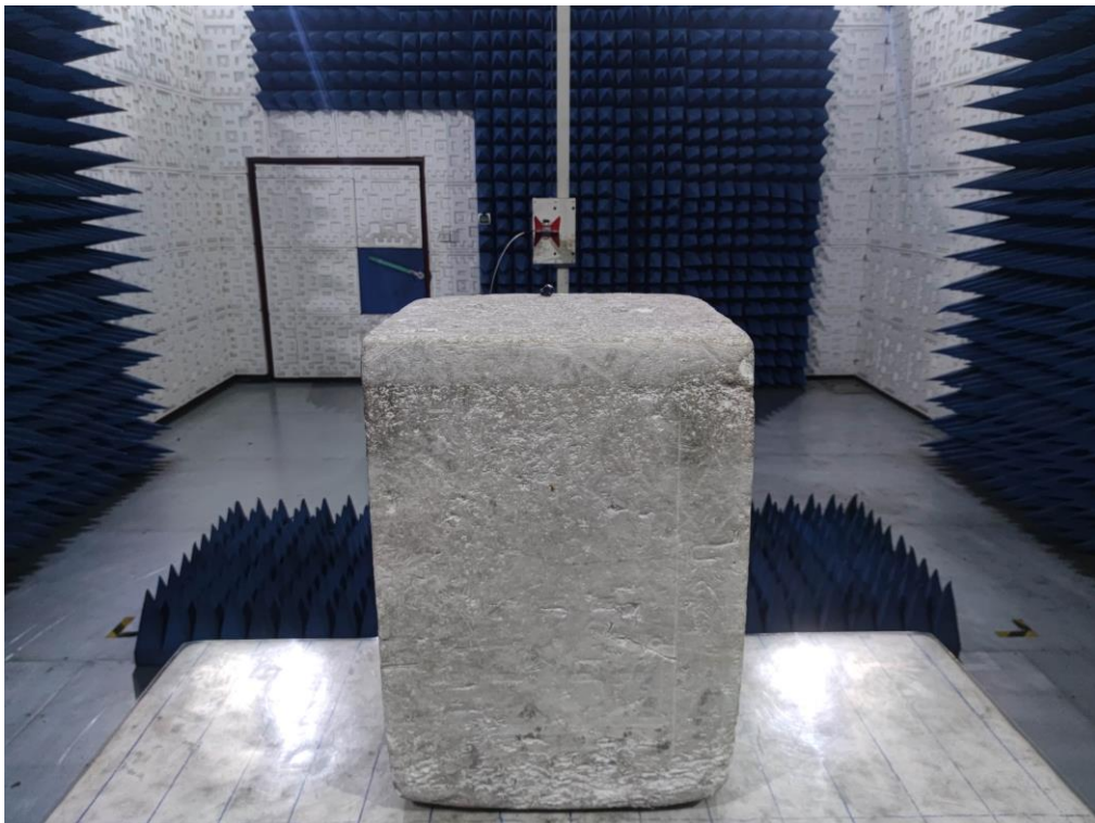
RADIATED EMISSION TEST SETUP ABOVE 1GHz
