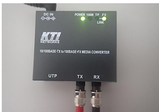
2-line fiber optics to LAN-TCP/IP converter.
