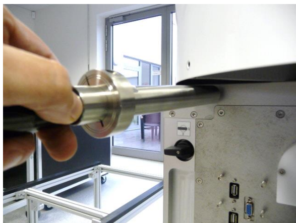
Use a wrench M19 to fix the handles firmly to the radar body.
