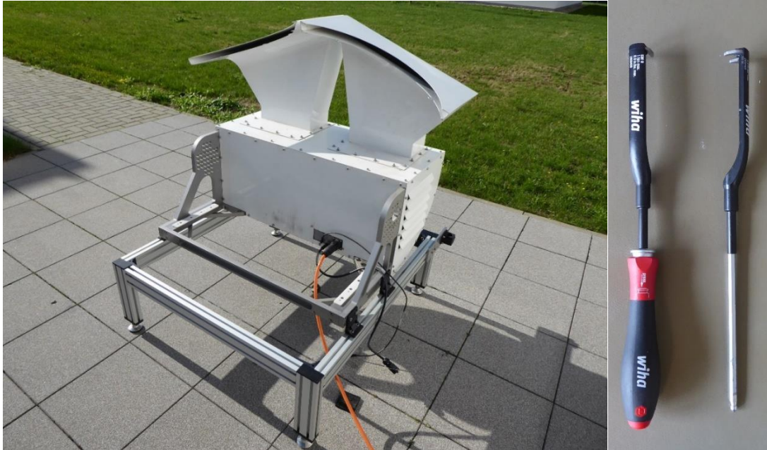
Left: The blower with air baffles and connected cables. Right: Tool to tighten the connectors.
