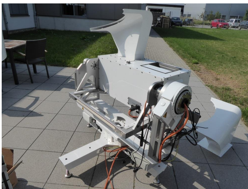
Unpacked scanner with one air baffle installed.
