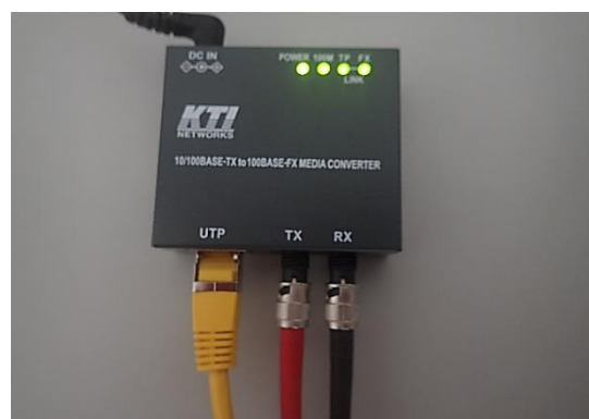
2-line fiber optics to LAN-TCP/IP converter.
