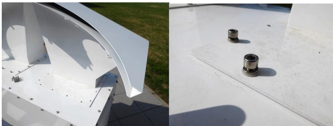
Do not tight the screws to make the installation of the radar body easier.
