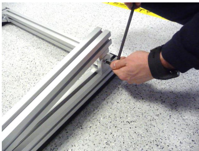
Use Allen key to release the screws.
