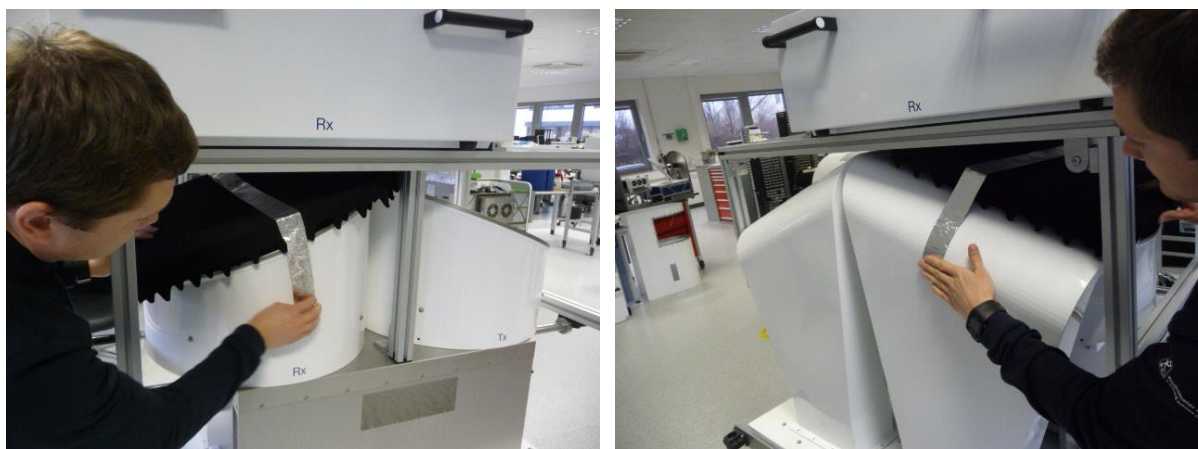
Mounting the ambient target.
