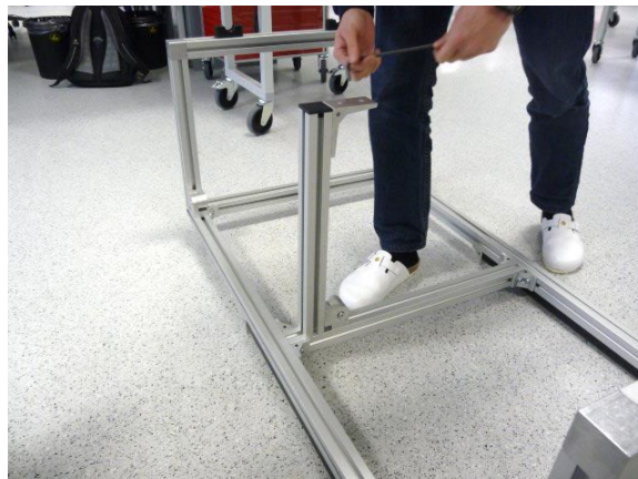
Tighten the screws when the frame has been unfolded.
