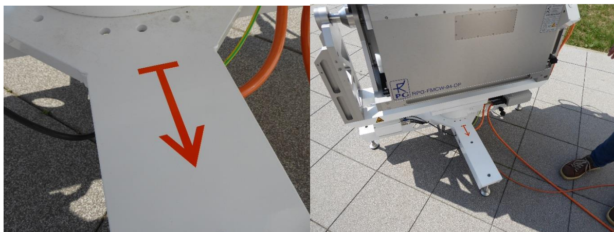
The arrow indicating 0° position of the scanner.
