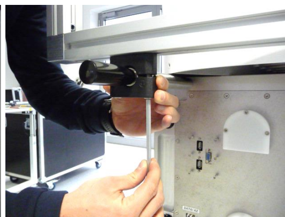
Mounting the frame to the radar housing.
