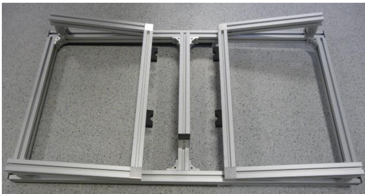
Frame for the LN2 target installation.
