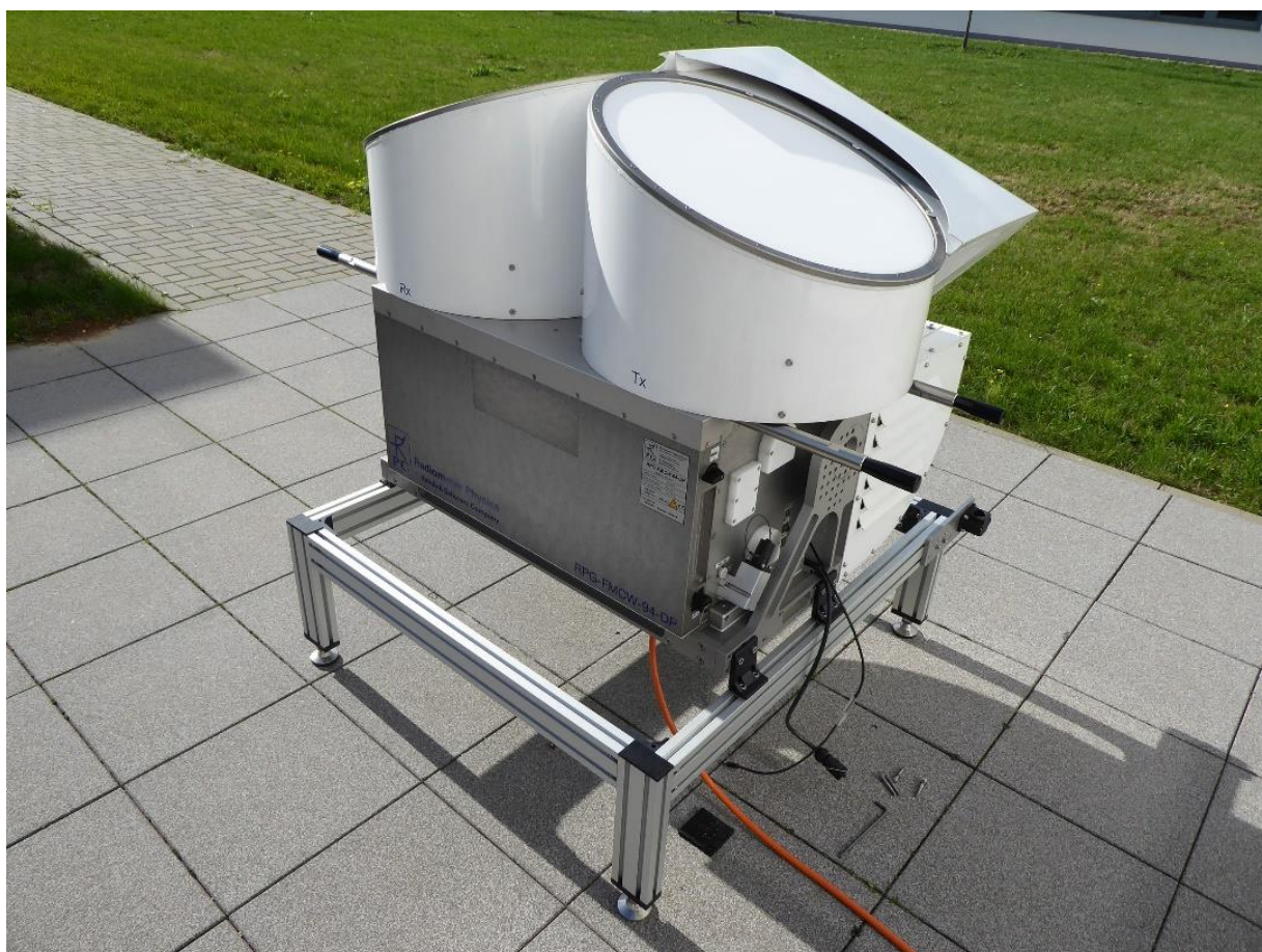
The radar body installed on the stand.
