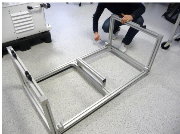
Tighten the screws when the frame has been unfolded.
