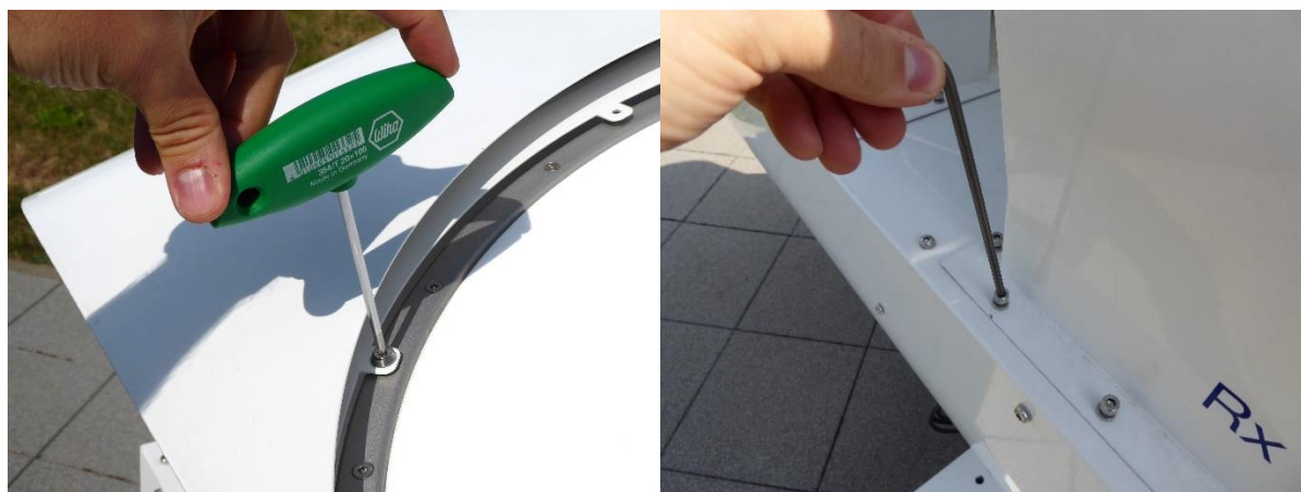
Unmounting the air baffles. Only use the T20x100 screwdriver (left) with the green handle and an Allen key (right)!
