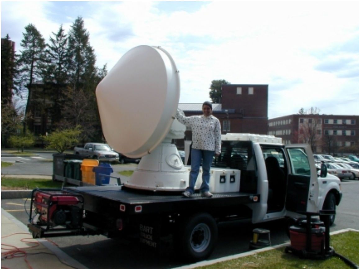
Figure 1. The UMass X-pol radar system with graduate student Vidhya Thyagarajan - the designer and programmer of the radar control and data acquisition system. The new radar will provide real time, long-range (60km +) images of storm structure to assist navigation during tornado chases.
