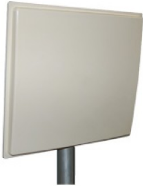
PA912: 15x15 inch High Gain Linearly Polarized 902-928 MHz Panel Antenna For ISM or RFID
