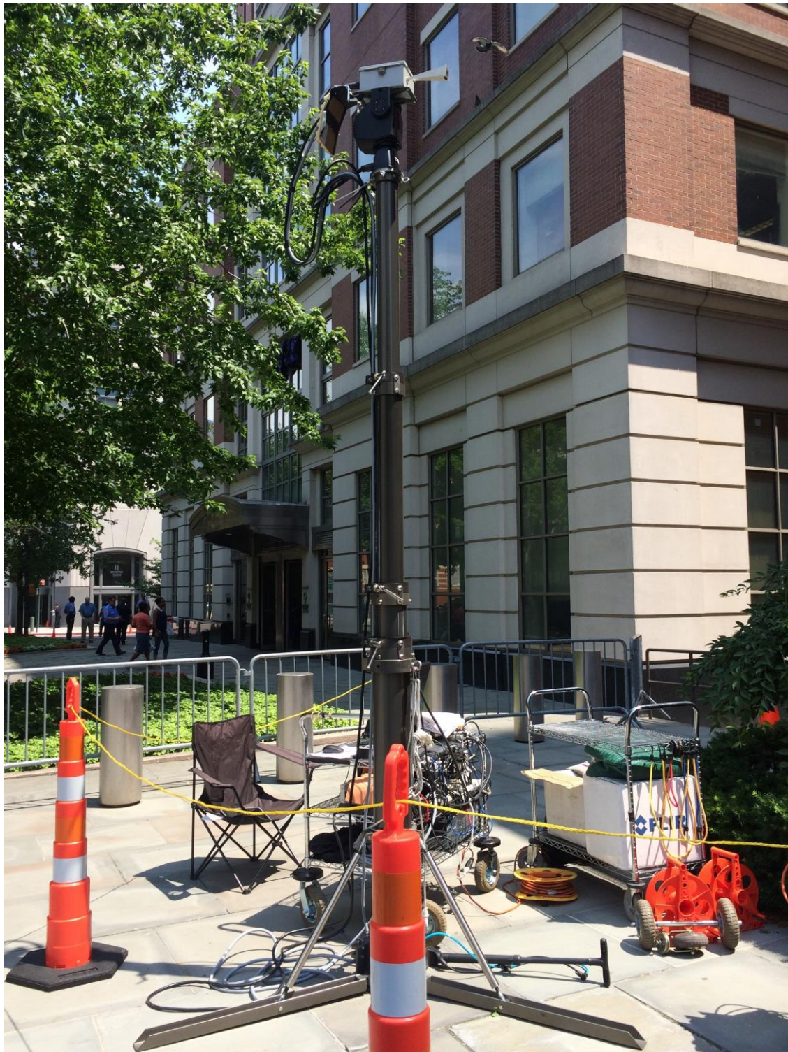
The transmitter cart and 4-m mast
