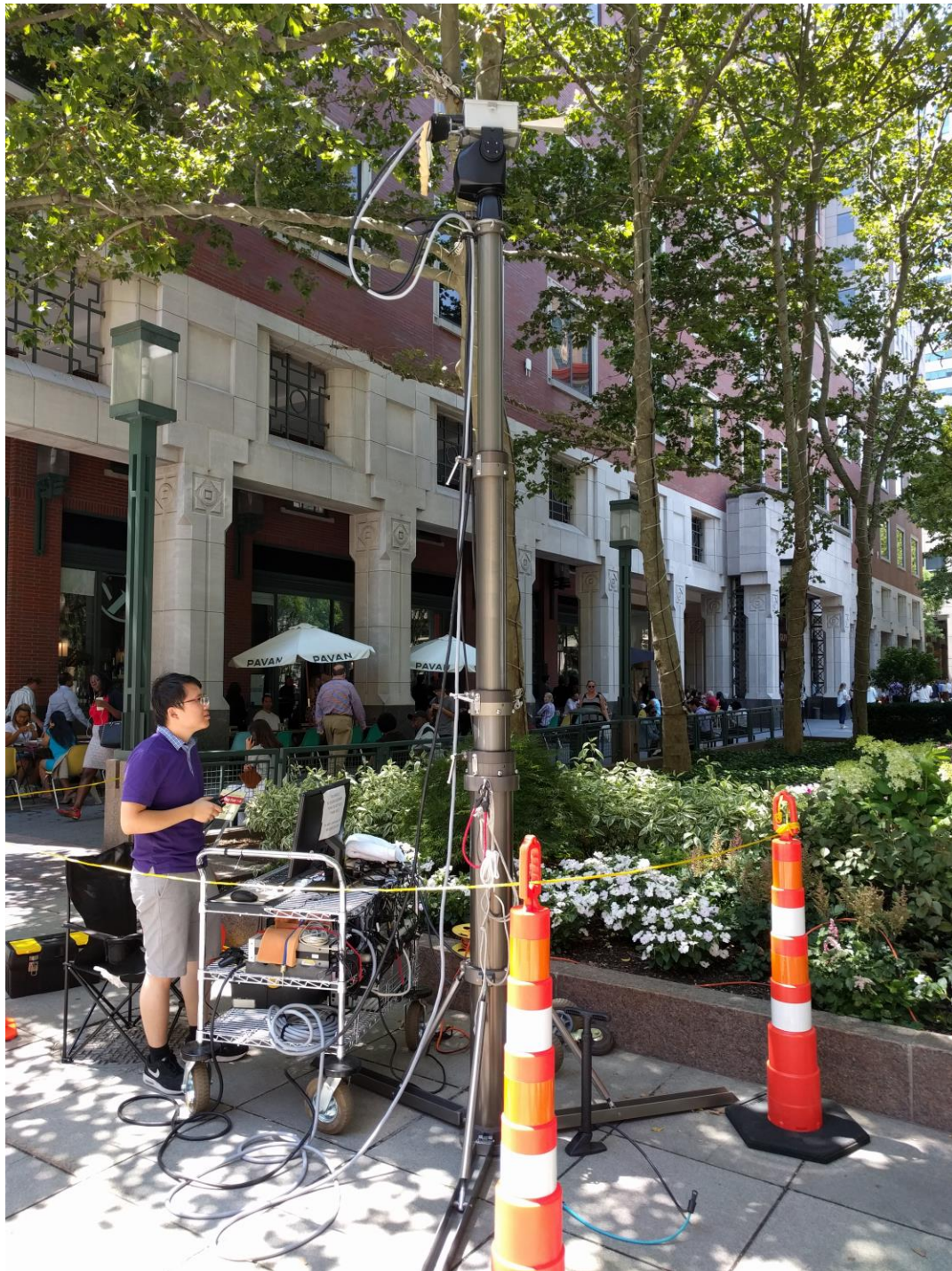
The transmitter cart and 4-m mast
