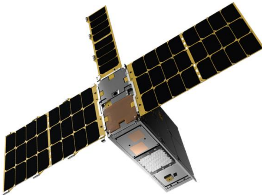
Figure 1: Cesium 6U spacecraft with solar panels deployed
