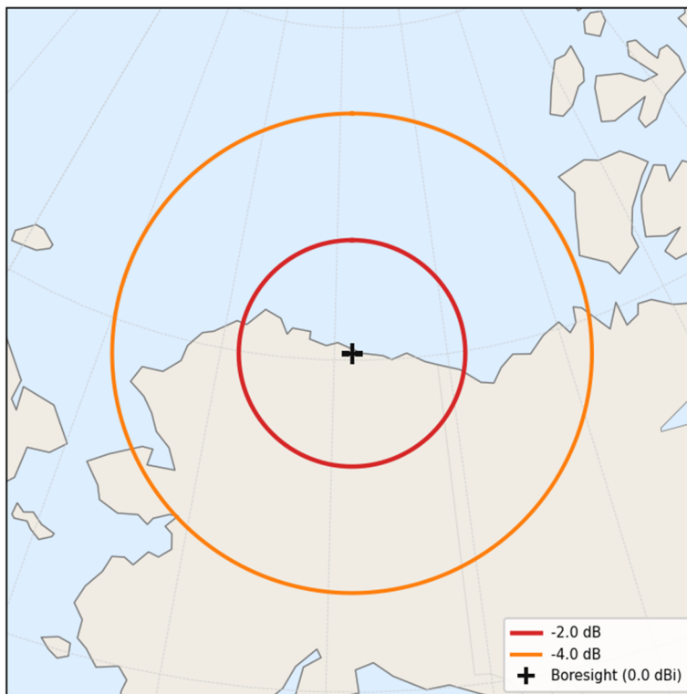
Figure 2 UHF receive uplink (URX) gain contours over Deadhorse, Alaska
