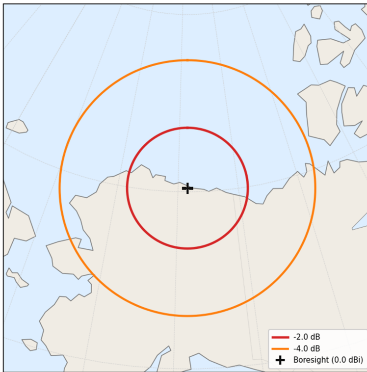
Figure 1 UHF transmit downlink (UTX) gain contours over Deadhorse, Alaska
