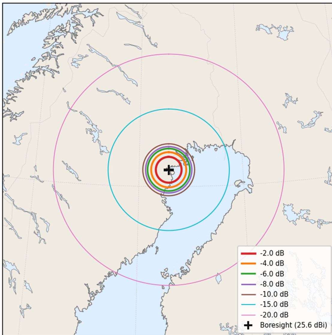
Figure 3.5 X-Band transmit downlink (XTX) gain contours over Boden, Sweden (350 km)
