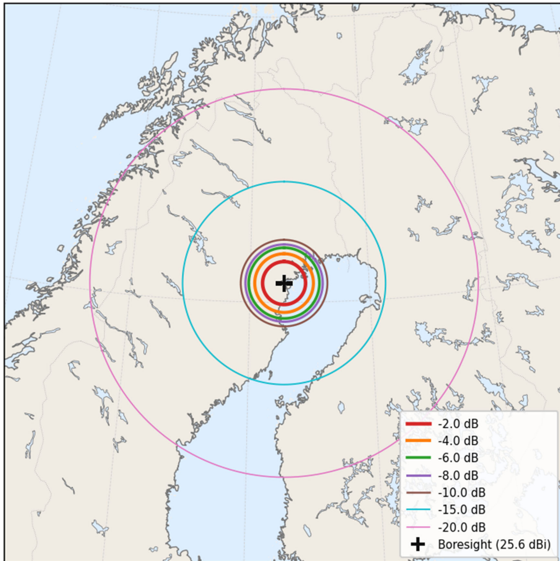
Figure 3.6 X-Band transmit downlink (XTX) gain contours over Boden, Sweden (510 km)
